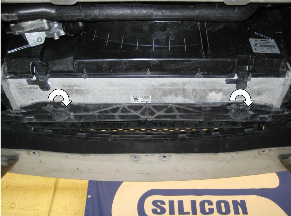
5. Using a T25 screwdriver, undo the screw on each side of the intercooler. Be sure to support the intercooler as you remove the screws as these are all that's holding it in place.
