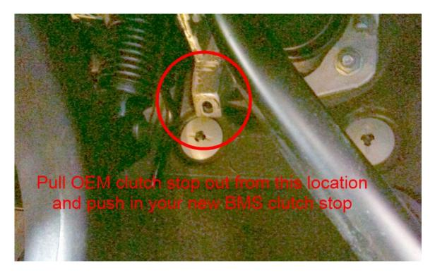
Push your BMS short throw clutch stop in its place until fully seated. For most applications all three adjustment shims are suggested. If you find the clutch throw too short for your taste you can remove shims as needed.
