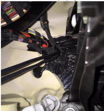
The wire will come out of an area behind the battery and can be run to the JB4 unit and plugged into the Molex plug.
