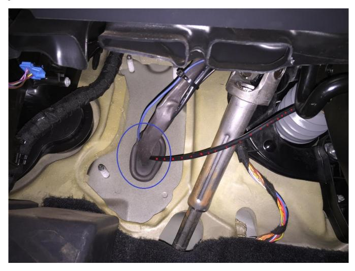
The OBD cable will exit behind the heat material on the firewall. Connect the plug inside the car and pull the cable so there is no slack left in the pedal compartment. This will allow for the cable to clear the steering column without rubbing.
