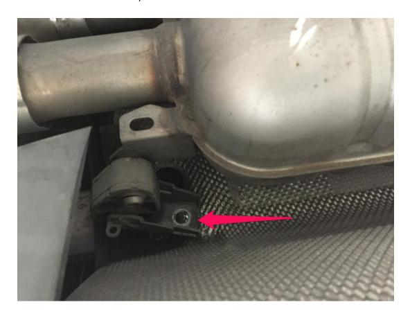
**Step 2** – Remove the triple square bolts securing the factory sway bar mounting brackets to the rear subframe.
