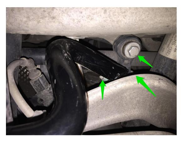
**Step 9** – Torque the sway bar end link hardware to 40 Nm + 90 Degrees. **Please Note:** We recommend replacing the factory end link bolts as they are torque-to-yield bolts.
