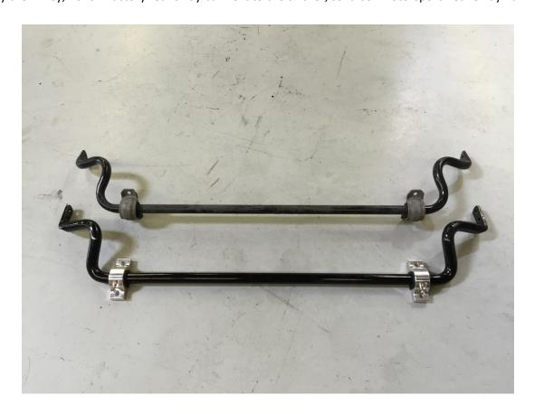
**Step 5** – Install the 034Motorsport Adjustable Solid Rear Sway Bar, noting the correct orientation below, and install the end links, loosely snugging up the hardware. **Do not fully tighten the end link hardware at this time!**
