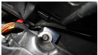
13. Remove these T30 torx on either side of the vehicle found just next to the light
