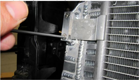
37. Pull the intercooler into the plastic cowling. There is a hole in the centre where your old bracket sat. Using the two screws provided, screw into the new brackets on your intercooler and tighten both sides .
