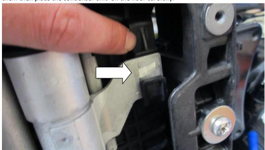
27. The radiator and intercooler are held in the cowling by these two clips. We found they broke when we tried to remove them, but don't worry we supply two new brackets that are screwed into position rather than clipped and will have been supplied with your new forge motorsport intercooler.
