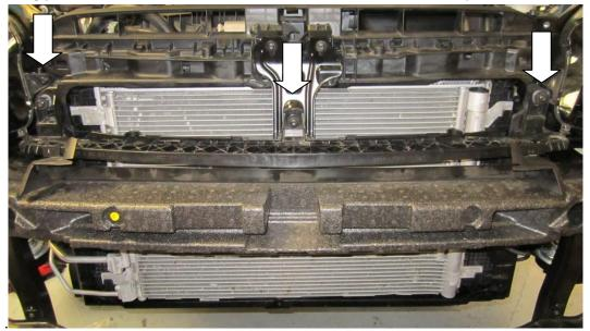
16. From underneath the vehicle you may now undo the pair of boost hoses on the OE intercooler
