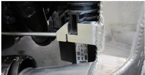
35. Place the new black plastic brackets on your intercooler to replace the old brackets. Two screws with washers are provided to hold these in position.
