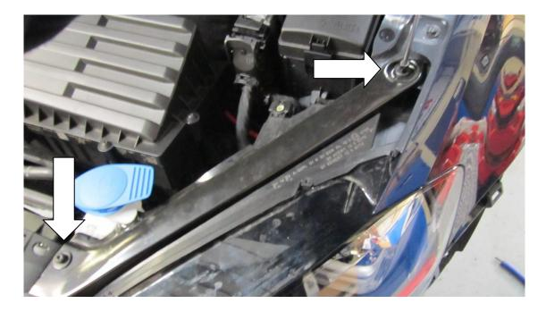
8. On the drivers side panel the bonnet catch housing is held on the underside. This must be disconnected, open the case and disconnect the cable .THIS MUST BE RECONNECTED ON REASSEMBLY OR YOUR BONNET RELEASE WONT WORK
