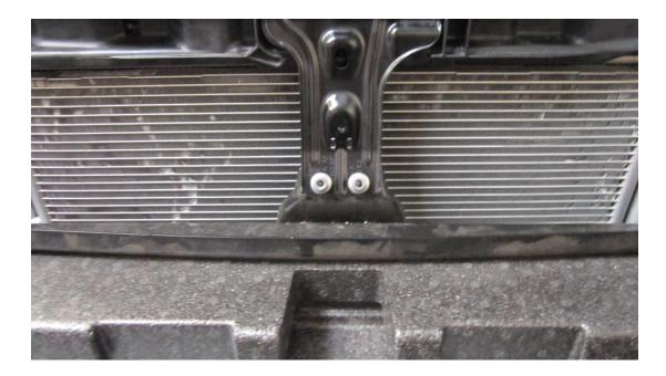
7. Using your T30 Torx drive undo the two fastners on either side of your car that cover the lights .
