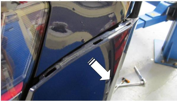
11. You may need some help lifting off the bumper as the wiring to the day time running lights must be disconnected. The washer bottle hose must also be separated. Get a clean container to catch the screen wash in if you wish to re-use as this will leak out once the hose is disconnected.
