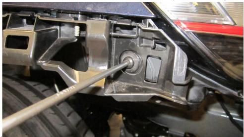
14. Disconnect your headlight wiring loom and remove your headlights from your vehicle.
