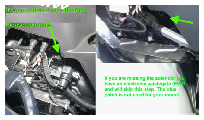
The solenoid is located under the engine cover. You'll lift it up to access the connection.
