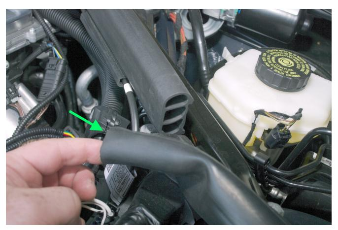
Now run the JB wire harness between the split in the weather seal and replace the weather seal as shown. The portion of the wire harness with the AMP cover on the connector should now be near the brake booster.
