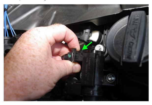
Lay the JB harness over the engine and locate the connector pair with blue wires. Plug the female connector on the JB N20 Stage 1 harness over the factory connection as shown, making sure that the retaining clip clicks into place. Then, plug the factory harness connection you removed in the last step onto the male connector on the JB harness, making sure that the retaining clip clicks into place.
