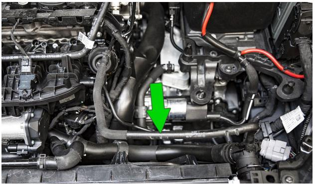
**15.** Using pliers, slide the coolant line hose clamps above the the coolant barbs on both ends, do not remove the coolant hose in this step.
