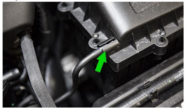
**4.** Use a pair of pliers or hose clamp pliers to remove the hose clamp from the airbox side of the turbo inlet hose and completely remove the airbox lid.
