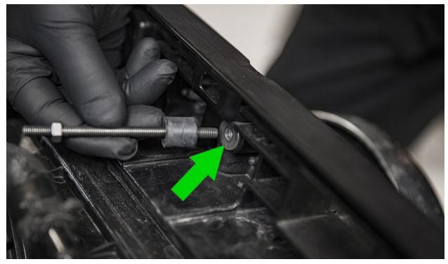
**35.** Place the complete intake assembly loosely into the car, carefully push down on the airbox to seat the grommet onto the factory plastic stud on the battery tray.
