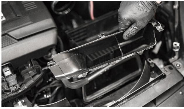
**11.** You can now remove the entire intake inlet box that spans the front of the car by pulling up on the lock tabs located on both corners.
