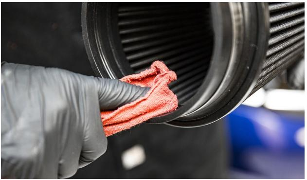
**24.** Install the air filter and clamp onto the velocity stack. Firmly tighten hose clamp with a screwdriver.
