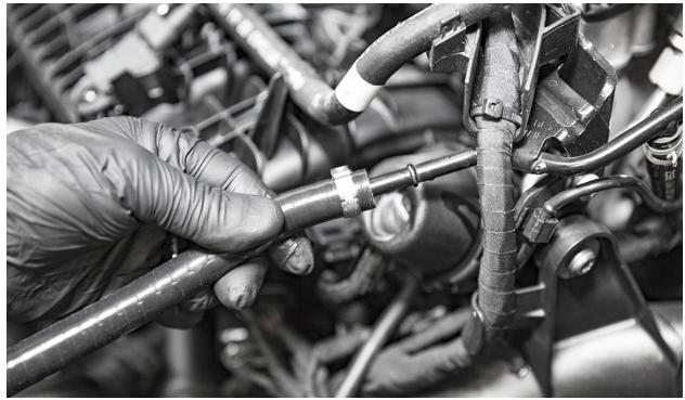
**19.** With the coolant line installed, tighten the pinch clamps using either the VW/Audi factory tool (if available) or wire cutters.
