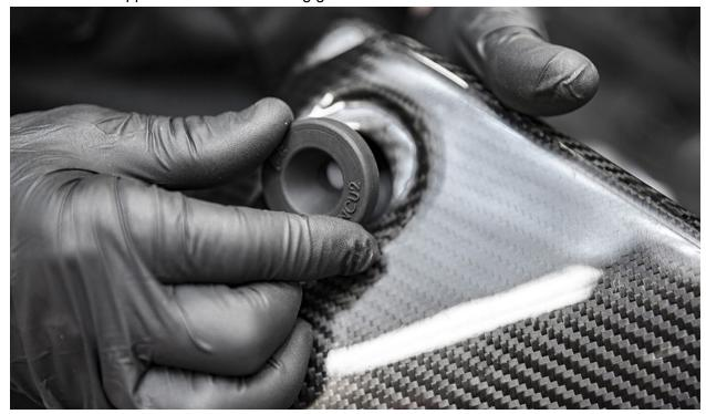
**28.** Carefully wipe down the underside of the intake inlet with a non-oily cleaner and allow it to dry. Remove the adhesive backing from the included foam square, and install it on the underside of the intake opposite of the IE logo plate as shown in the photo below. Make sure the foam is placed correctly, once installed it is permanent.
