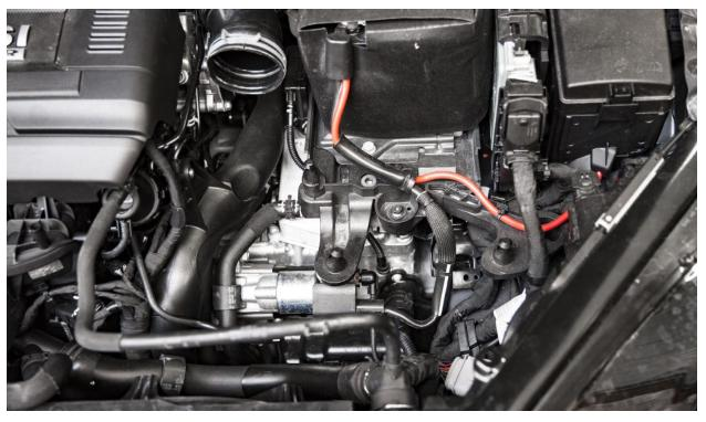
**13.** Remove the engine factory cover by pulling up on the two sides firmly.
