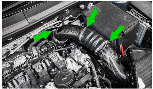
**43.** If you do not have the carbon turbo inlet pipe, install the factory plastic turbo inlet onto the assembled airbox using the factory clamp.
