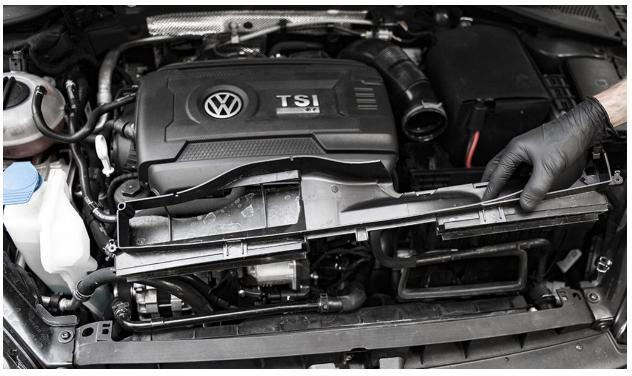
**12.** Carefully pull up on the factory lower airbox to release it from the battery tray and remove it. The airbox is held in place on the underside by 3 rubber grommets securing it to plastic posts.
