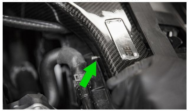
**38.** Using your hands, adjust the intake to remove the gap between the intake and radiator so that the intake sits flush and consistent across the front of the vehicle. Note the placement of the intake on the stud in this position.
