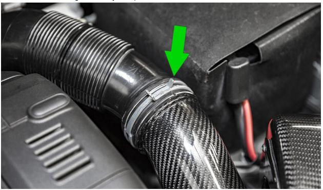
**44.** Install the factory vacuum hose onto the 90 degree barb fitting located on the underside of the velocity stack inlet.
