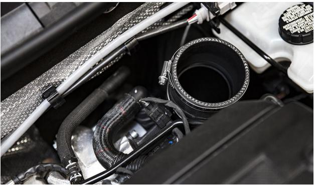
**32.** Install the silicone hose and hose clamps onto the carbon turbo inlet pipe. Do not tighten the hose clamps in this step. You may find it helpful to use a non oily lubricant, such glass cleaner to install the silicone. The silicone coupler should be positioned so it points towards the turbo.
