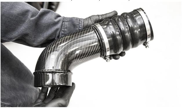
**33.** Now install the silicone coupler and carbon turbo inlet pipe onto the assembled carbon airbox, leaving the clamps loose.
