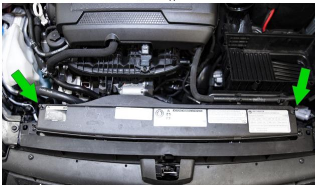
7. Pull to release the tab on the back side of the upper airbox inlet cover, then fully remove it.
