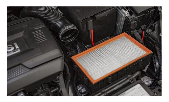
**5.** Remove the air filter by simply pulling it out.
