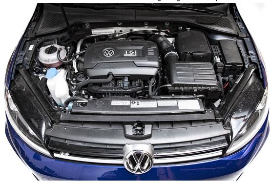
**2.** Start the installation procedure by loosening the eight T25 bolts from factory airbox lid. These do not fully remove, just loosen them until they are spinning freely.
