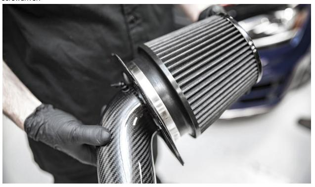
**25.** Install the carbon fiber velocity stack and air filter onto the carbon airbox. The pre-installed 90 degree vacuum barb on the velocity stack should be aligned with the bottom side of the air box.
