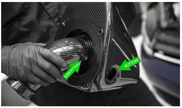
**26.** Using a 3mm allen wrench, tighten the four included 3mm socket head bolts to secure the velocity stack to the airbox. Do not over-tighten as it can crack or warp the carbon fiber.
