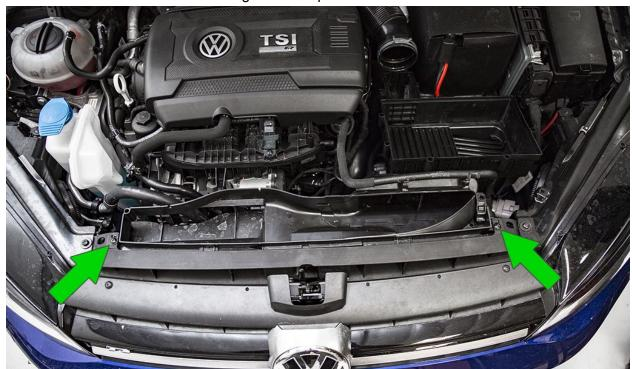
**10.** Remove the end section of the intake inlet box (shown below) located in front of the airbox by pulling up on the lock tab.
