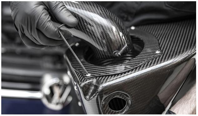
27. Install the supplied IE rubber mounting grommet into the bottom of the airbox.
