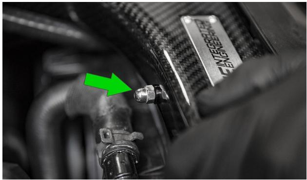
**41.** If you do not have the optional turbo inlet pipe, skip to step 43. Insert the turbo inlet pipe into the installed turbo silicone coupler. Re-align the turbo inlet pipe, and silicone hump coupler positions so everything sits in place relaxed without tension.
