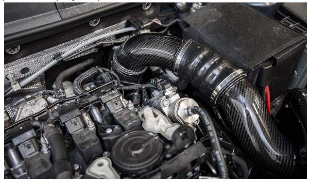
**42.** With the complete intake assembly properly positioned, tighten the 3 remaining hose clamps.
