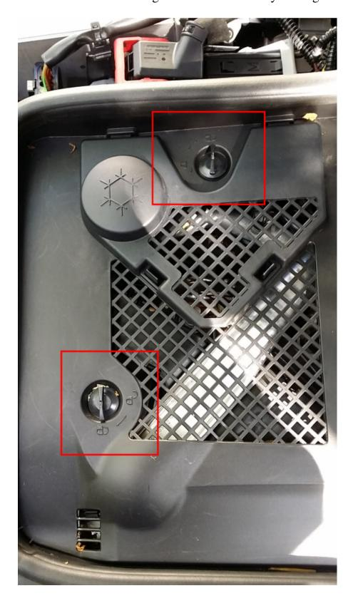
Tuck the wiring harness with control box attached under the plastic cover behind the brake booster as shown. You can secure the box to the brake booster area with a zip-tie, or simply wedge it between the brake booster, and the engine cover. Care should be taken to ensure the box is not left under the grated area of the engine cover where water could drip in to the control box.
